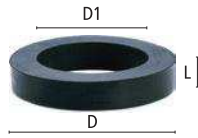
O-ring made of NBR 55° Shore A
