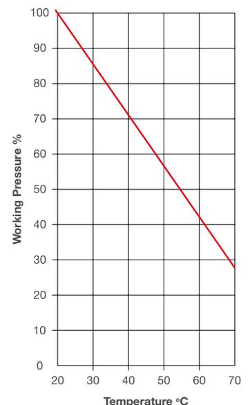
Max. recommended continuous working temperature = 60°C
